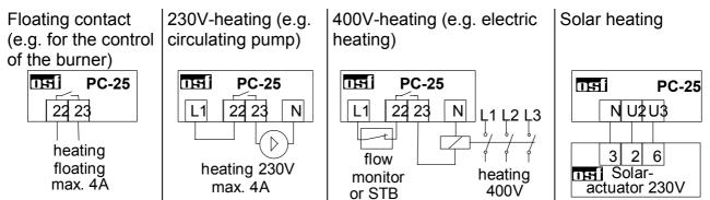
The floating relay contact between the clamps 22 and 23 can be charged with a maximum voltage of 230V with maximum 4A.
