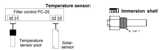
The pool temperature sensor is connected to the clamps 30 and 31. As a standard the temperature sensor is delivered with cable length of 1.5m. If required, this can be lengthened with a two-core cable (minimum diameter 0,5mm<sup>2</sup>) up to a maximum of 20m. It should be avoided to lay the sensor lead near power lines to exclude possible disturbance.
