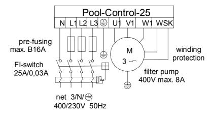
The factory-provided inserted bridge between the two clamps called WSK, has to be removed, if connected with a pump with winding protective contact. If no connection is carried out, it has to be remained screwed in. The clamps drive mains voltage!
