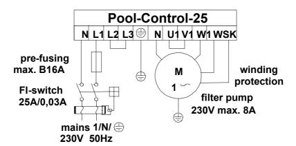
Mains supply for use of a 230V-alternating current pump:
