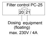
In the control unit there is a floating relay contact between the clamps 20 and 21. This can for instance be used to control the dosing equipment (the contact will be closed during the filter operation). This contact can be charged with a maximum of 230V/4A.
